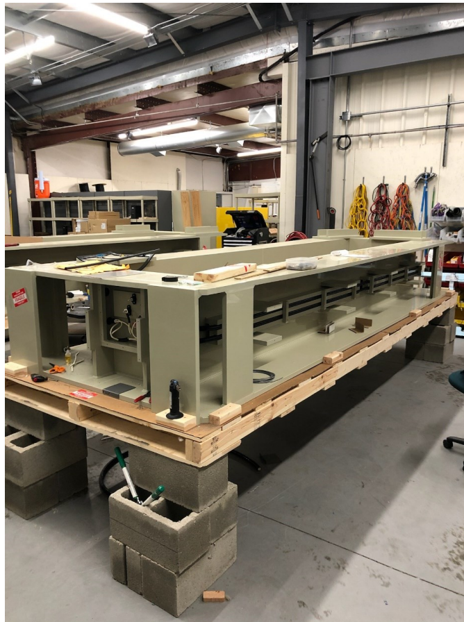
Figure 2. Washington Shore serpentine weir replacement antennas under construction at the PTAGIS Kennewick Lab.
