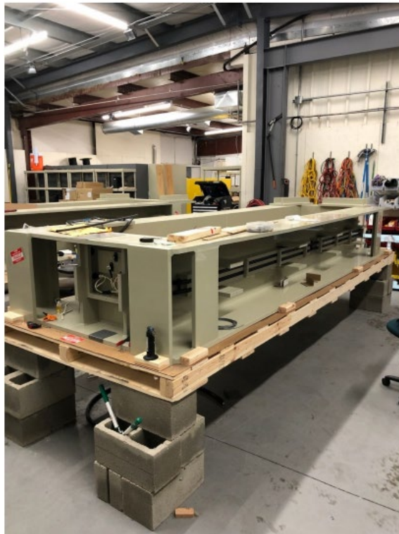
Figure 19. New BO4 PIT tag antennas under construction at the Kennewick lab.
